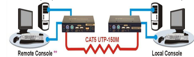
LKV-E235 CAT5 KVM Extender Configuration Diagram
