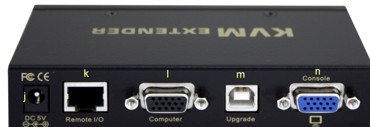
Transmitter (Tx) Unit – Back Panel [Directly connected to the 1 st computer]
