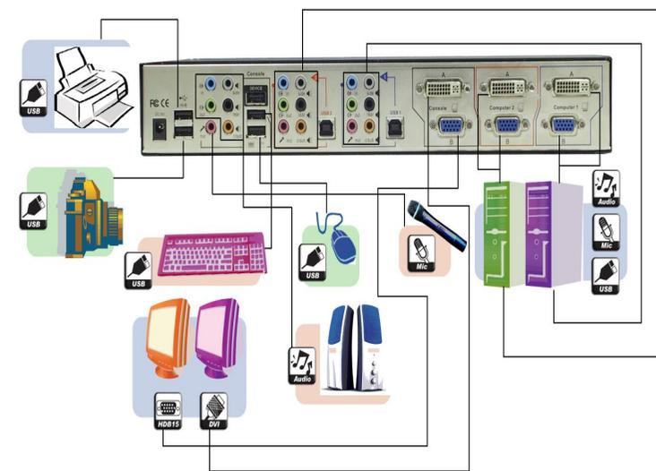
Basic configuration (showing only LDV-DM712AUSK)
